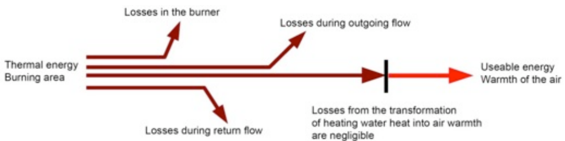
Pic 3.3:Flow of energy in gas heating
