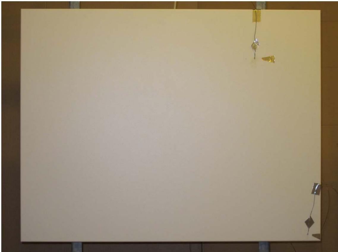
**Figure 3:** Front side of the radiation heater with two temperature sensors
